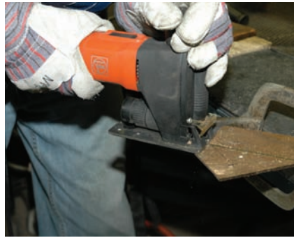
Let the saw do the cutting, very little pressure is necessary to make a smooth line.
