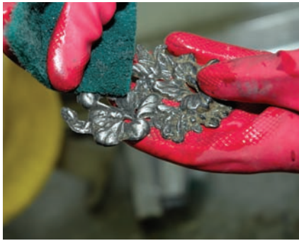
Lightly brush blackening off the pewter casting with a scrub sponge. Details will be highlighted.
