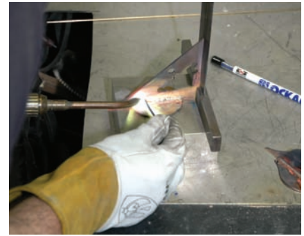
Do not melt the braze with the torch, it should melt on contact with the joint.
