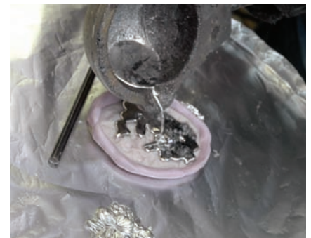
For best results, dust all moulds with talc powder and pour pewter slowly.
