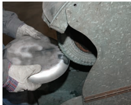
In order to get an even finish, buff in the same direction.
